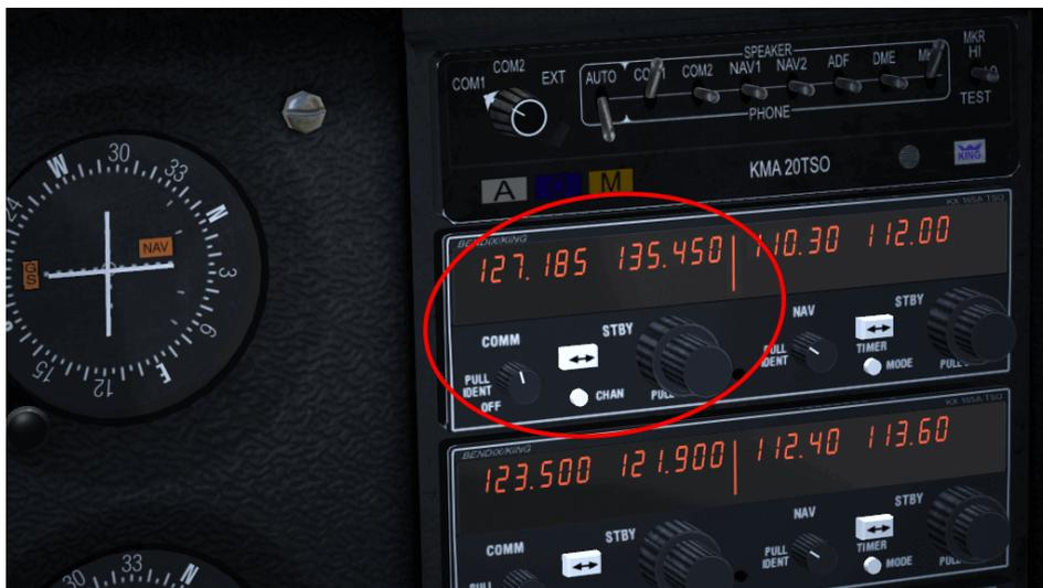
Figura 9.4: The C172 communications stack with COMM1 highlighted
