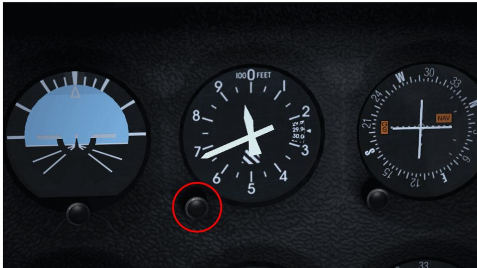
Figura 9.8: Altimeter calibration knob
