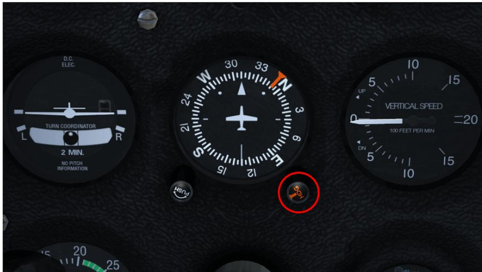
Figura 9.9: Heading adjust knob
