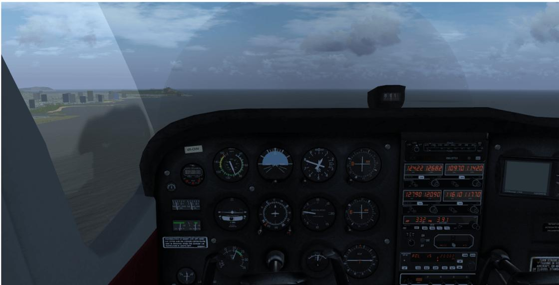
Figura 8.14: Straight and level flight
