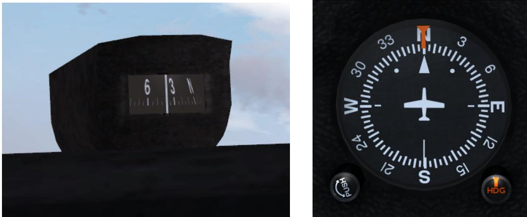
Figura 8.28: Magnetic compass & heading indicator
