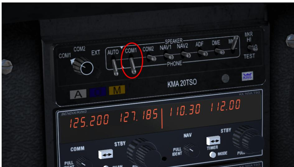
Figura 9.7: Speakers switch for COMM1
