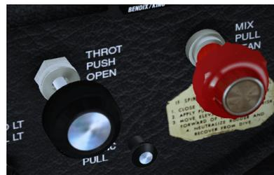
Figura 8.23: Throttle & mixture
